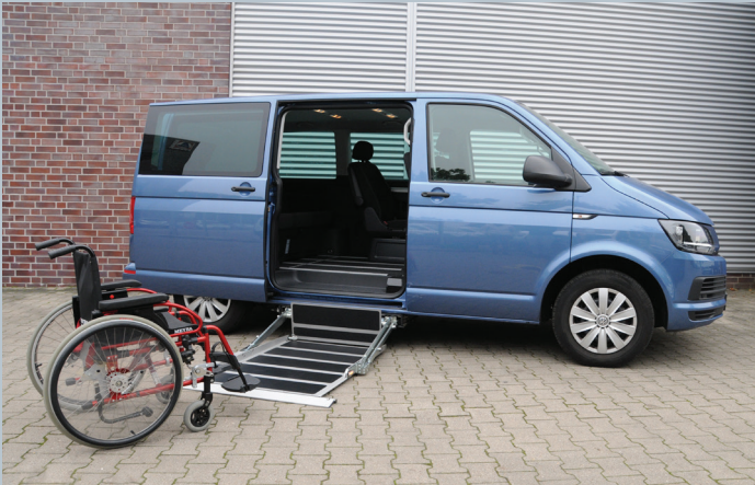
The lateral access option with the flat side edge of the lifting platform saves space when driving up with the wheelchair.
