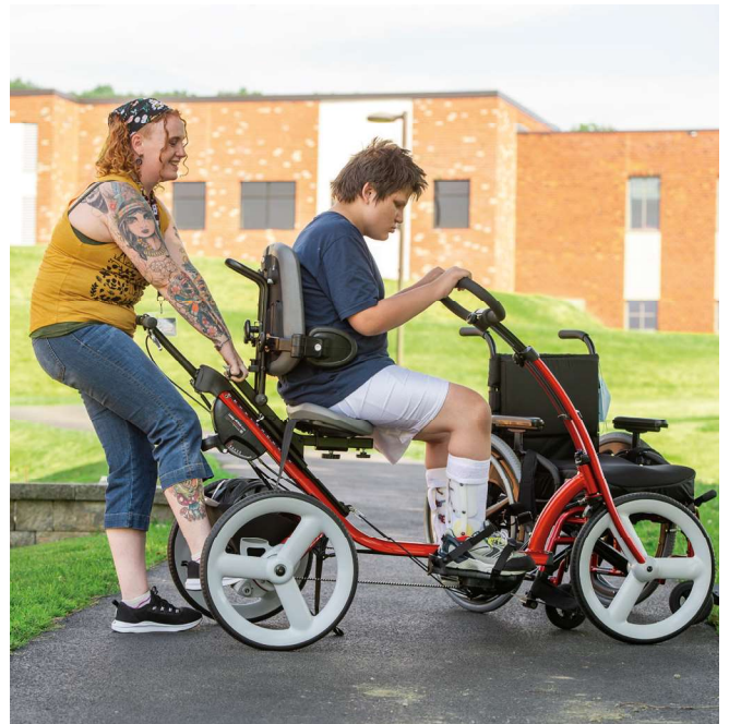
The seat glides up and down on a low-friction rail. This rider pushes with his feet to help his caregiver raise the seat.
