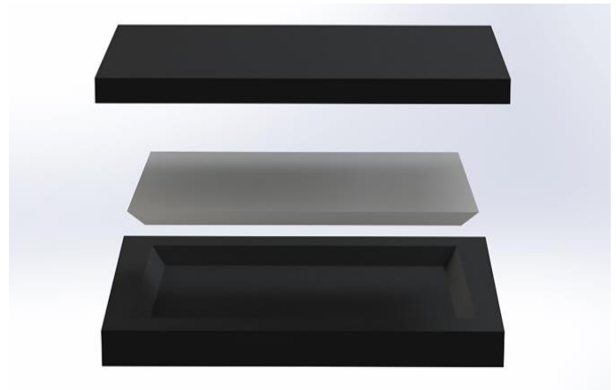
The seat cushion is made up of three different types of foam.
