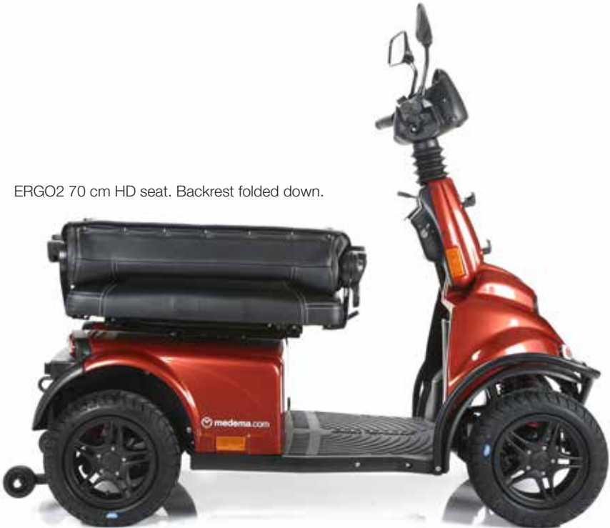
Seat angle The seatback angle can be adjusted 45° backwards and 90° forwards. This is done by pulling the handle on the right side of the seat.
