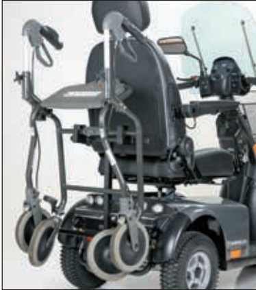
1506-1281 - Rollator carrier, max. weight 20 kg (44lb).
