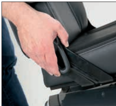
Seat angle The seatback angle can be adjusted 45° backwards and 90° forwards. This is done by pulling the handle on the right side of the seat.
