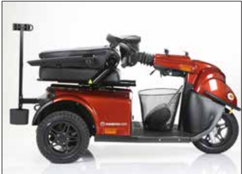
ERGO2 45 cm seat. Seat 180 degrees turned. Backrest folded down. With stick holder.
