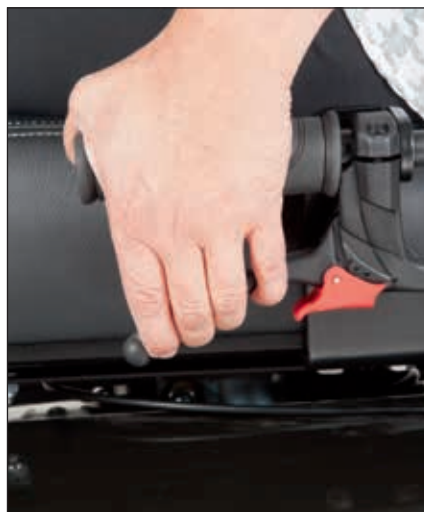
As an option, the Mini Crosser X-Joy can be equipped with a parking brake.
