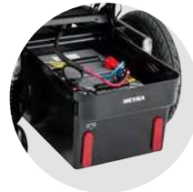
Easy battery maintenance thanks to pull-out battery case
